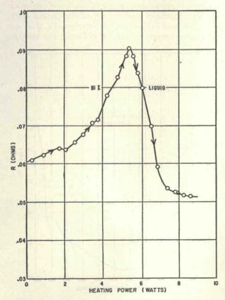
Fig. 6. Resistance change upon melting Bi I at 7800 kg/cm<sup>2</sup>.
