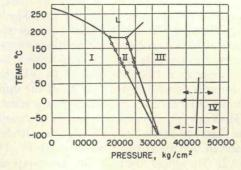
Fig. 1. Phase diagram of Bi (Bridgman).
