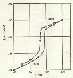
Fig. 8. Resistance change associated with Bi II → liquid.
