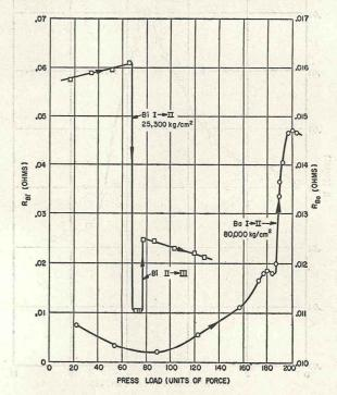
Fig. 10. Pressure calibration of cell by Bi and Ba transitions.
