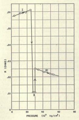
Fig. 7. Resistance changes associated with Bi I-II and Bi II-III at 25°C.
