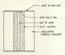
Fig. 2. Simple directly heated cell.
